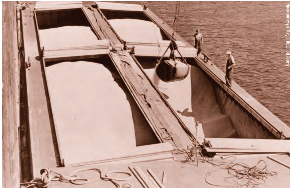
An all-steel barge constructed especially for hauling bulk wheat from the Inland Empire lays at Terminal 4 on the Willamette, waiting to discharge its 18,000-bushel load (ca. 1939).
